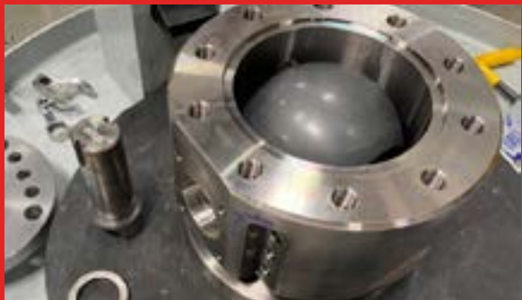
*Monel Severe Service Ball Valve Assembly
